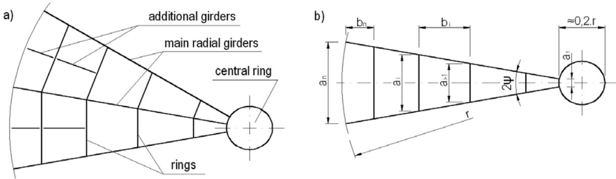
Fig. 1 Structure of the self-supporting roof
