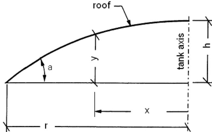
Fig. 4 Coordinates of dome roof
