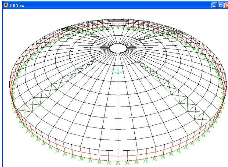
Fig. 3 Spatial frame model of the roof
