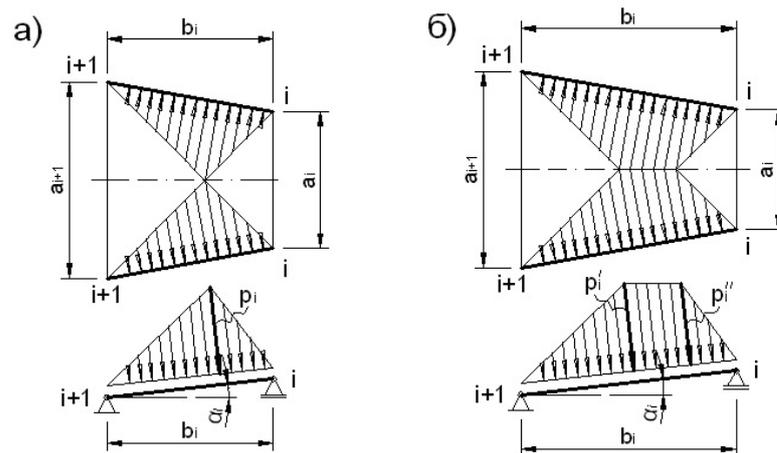
Fig. 2 Scheme of loads on the radial girders
