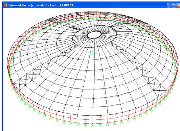
Fig. 4 Deformed shape of dome roof , that loses stability, due to loading of self weight  $g_n$  and vacuum  $p_v^n$
