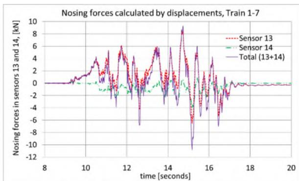
d) nosing forces from train 1-7, accounted by displacement of sensors №13 and №14
