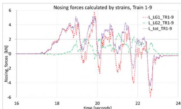
f) nosing forces from train 1-9, accounted by strains in flanges of longitudinal beams
