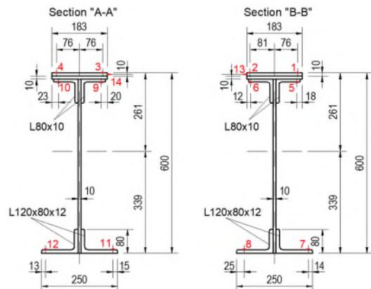
Figure 4. Sections of the longitudinal girders and points of placement of the strain sensors
