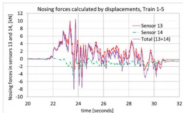
b) nosing forces from train 1-5, accounted by displacement of sensors №13 and №14
