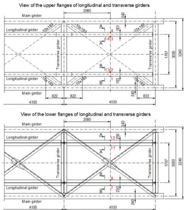
Figure 3. Main dimensions of the deck structure of the bridge and points of placement of the sensors
