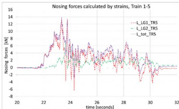
b) nosing forces from train 1-5, accounted by strains in flanges of longitudinal beams
