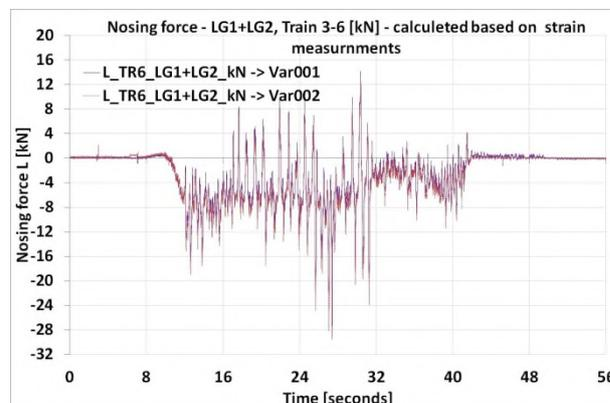
Figure 9. Nosing forces in both longitudinal beams of the bridge, due to freight train 3-6
