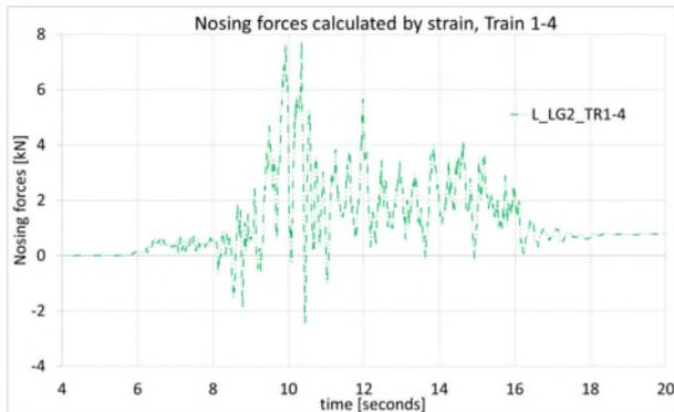
a) nosing forces from train 1-4, accounted by strains in flanges of longitudinal beams
