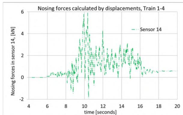
a) nosing forces from train 1-4, accounted by displacement of sensor №14
