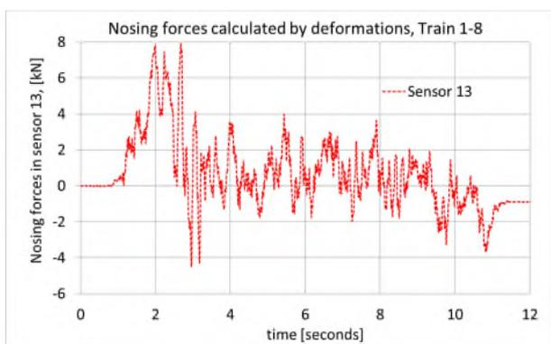
e) nosing forces from train 1-8, accounted by displacement of sensor №13
