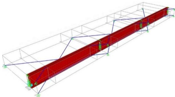
Figure 5. A numerical model of longitudinal girders
