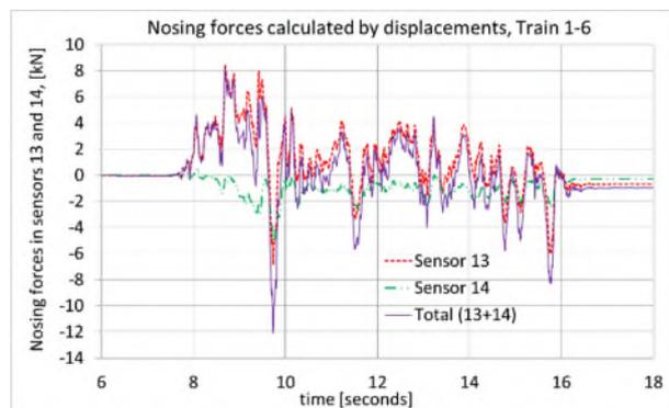
c) nosing forces from train 1-6, accounted by displacement of sensors №13 and №14
