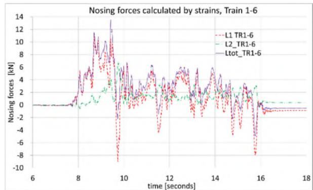
c) nosing forces from train 1-6, accounted by strains in flanges of longitudinal beams
