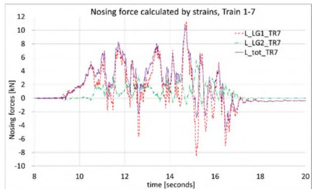
d) nosing forces from train 1-7, accounted by strains in flanges of longitudinal beams
