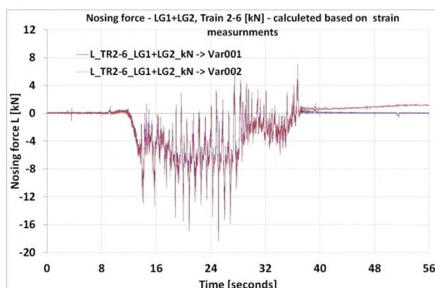
Figure 8. Nosing forces in both longitudinal beams of the bridge, due to freight train 2-6
