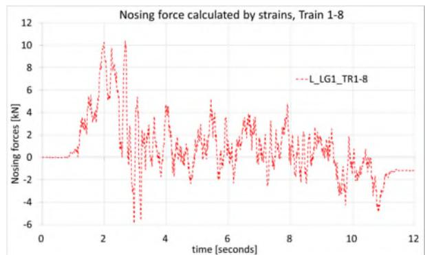
e) nosing forces from train 1-8, accounted by strains in flanges of longitudinal beams
