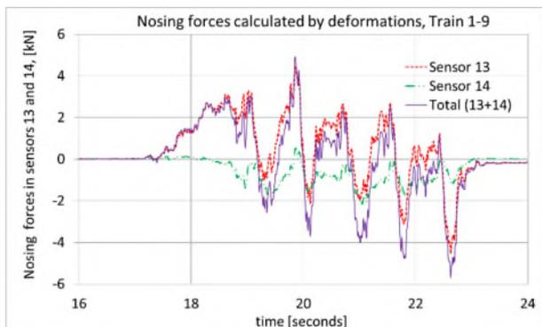
f) nosing forces from train 1-9, accounted by displacement of sensors №13 and №14
