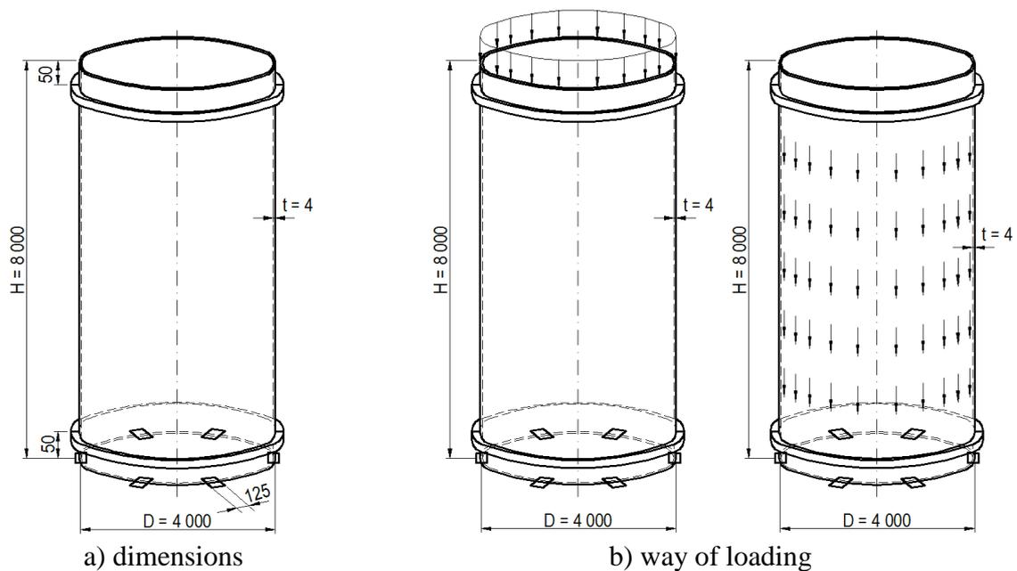
**Fig. 1** – Numerical model – dimensions and ways of loading
