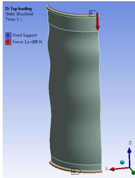
**Fig. 3** – Loading on part of symmetrical shell with imperfections
