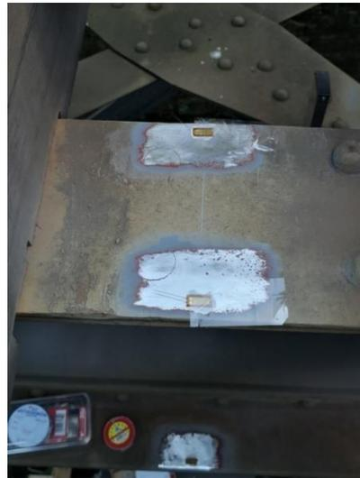
b) glueing of strain gauge sensors
