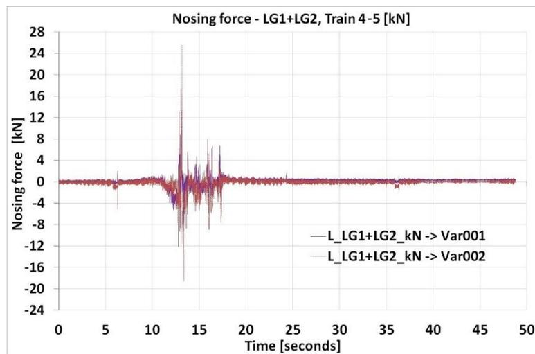
**Fig. 6. Nosing forces due crossed passenger train 4-5**
