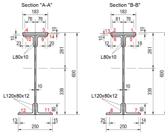
Fig. 3. Sections of the longitudinal girders and points of placement of the strain sensors
