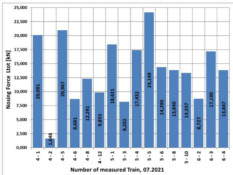
**Fig. 8. Total value of nosing forces in the two longitudinal beams of the bridge, accounted by the strains in the flanges of the beams**
