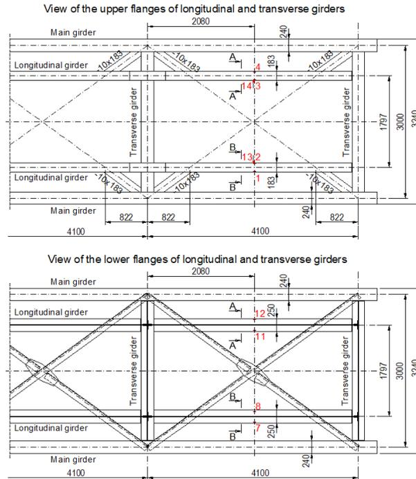
**Fig. 4. Main dimensions of the deck structure of the bridge and points of placement of the sensors**
